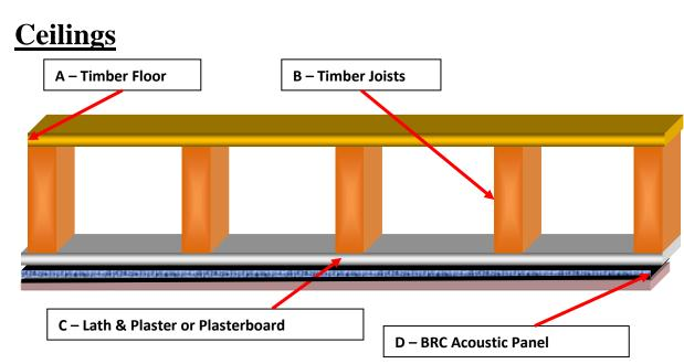
The Acoustic Panel is simply mechanically fixed over the existing ceiling and fixed to the ceiling joists using suitable screws. All abutments are sealed with Fire & Acoustic Sealant. The panel can then be painted or skimmed with plaster depending on the finish required.
